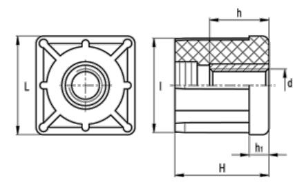
$\begin{array}{lll} d & = M12 \\ h & = 10 \\ H & = 38 \\ h1 & = 8 \\ Internal tube size = 35.0 \\ I & = 35.0 \\ L & = 40 \\ \end{array}$
